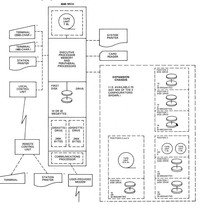
Figure 1. XL40 System Block Diagram
